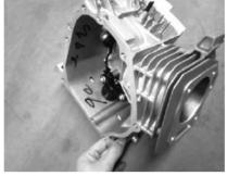
The oil alarm is designed to operate with a level engine (the working angle of the device with respect to the ground is usually less than 20°). If the motor has an inclination greater than 20°, then it will stop.
