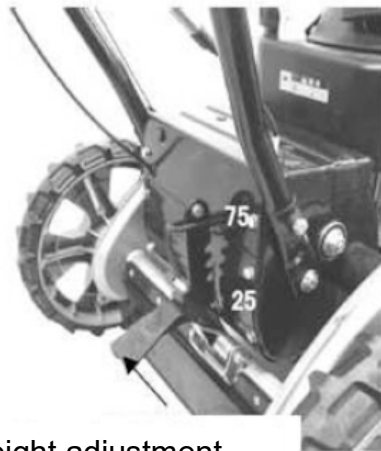
Rear wheel height adjustment
