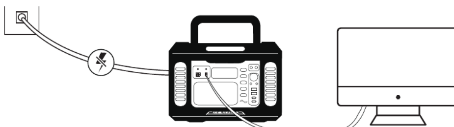
Operation specified for EPS mode.
