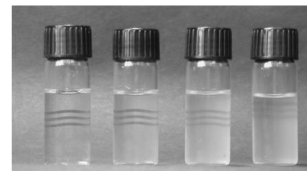
NOTE: This kit detects oil by forcing it to form bubbles. Familiarity with the results will enable the user to accurately estimate the oil / petrol ratio. It is recommended that new users test a known sample to use as a reference.
